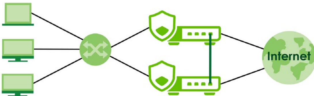
Figure 95 Device HA Backup Taking Over for the Master
